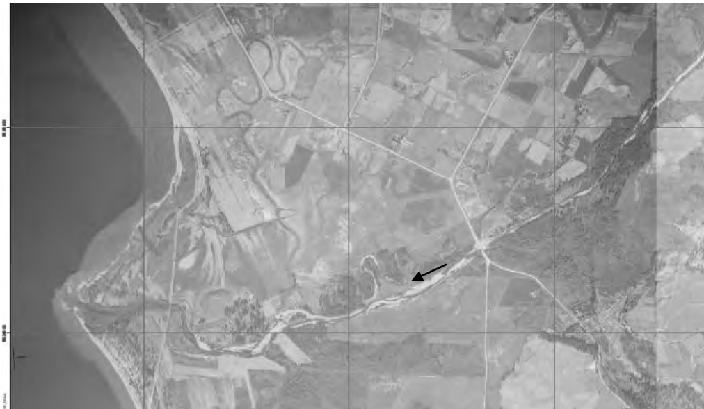
Figure 2-7. 1938 Mission Creek channel displaying the abandoned channels on the floodplain near KLO road. Arrows indicated flow direction.
