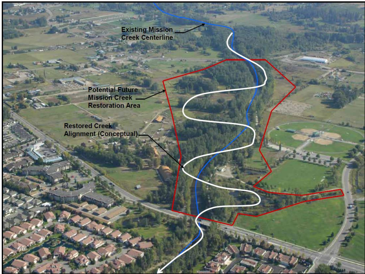
Figure 3: Conceptual Meandering in a Segment of Mission Creek Between Casorso Road and Gordon Drive
