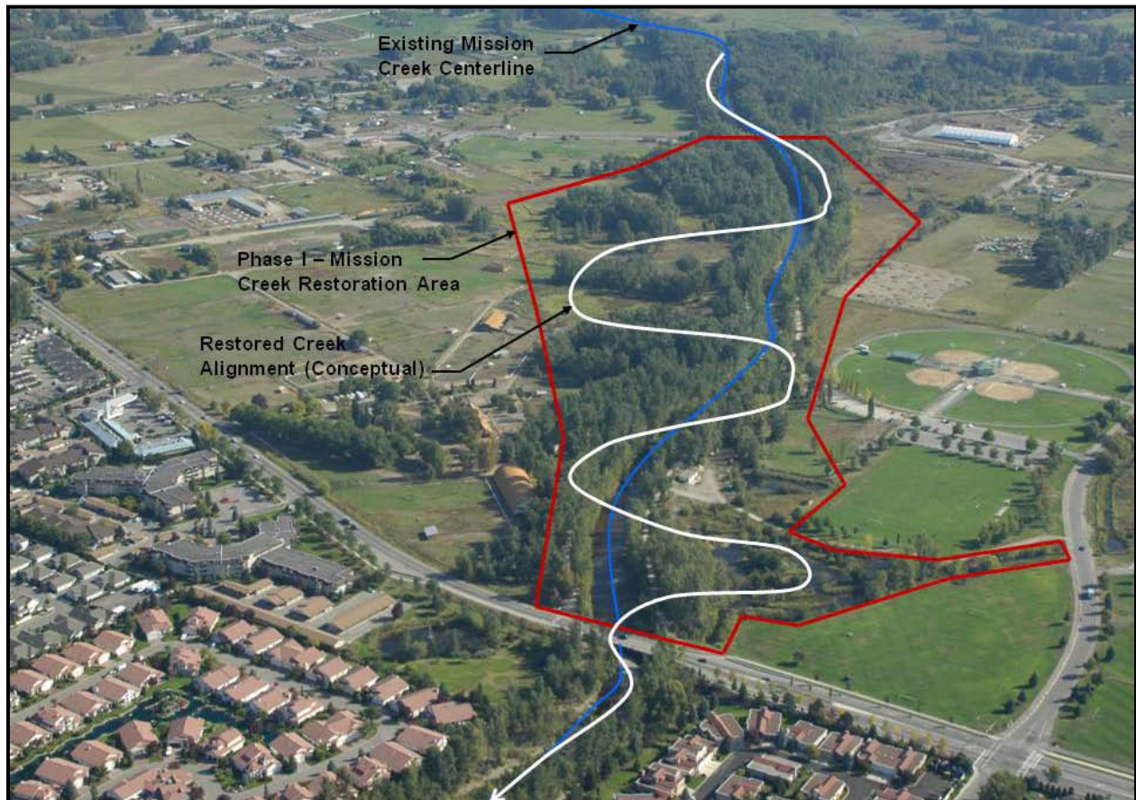
Figure 3: Phase I Restoration Area With Conceptual Re-meandering
