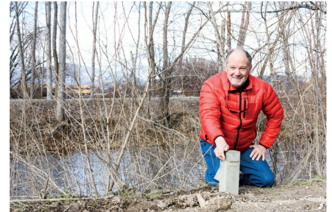
Project engineer Don Dobson identifies one of four monitoring wells that will help determine if the new dike impacts ground water levels over time.
